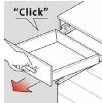
Pull out sharply HORIZONTALLY until the drawer audibly disengages and then lift off.
